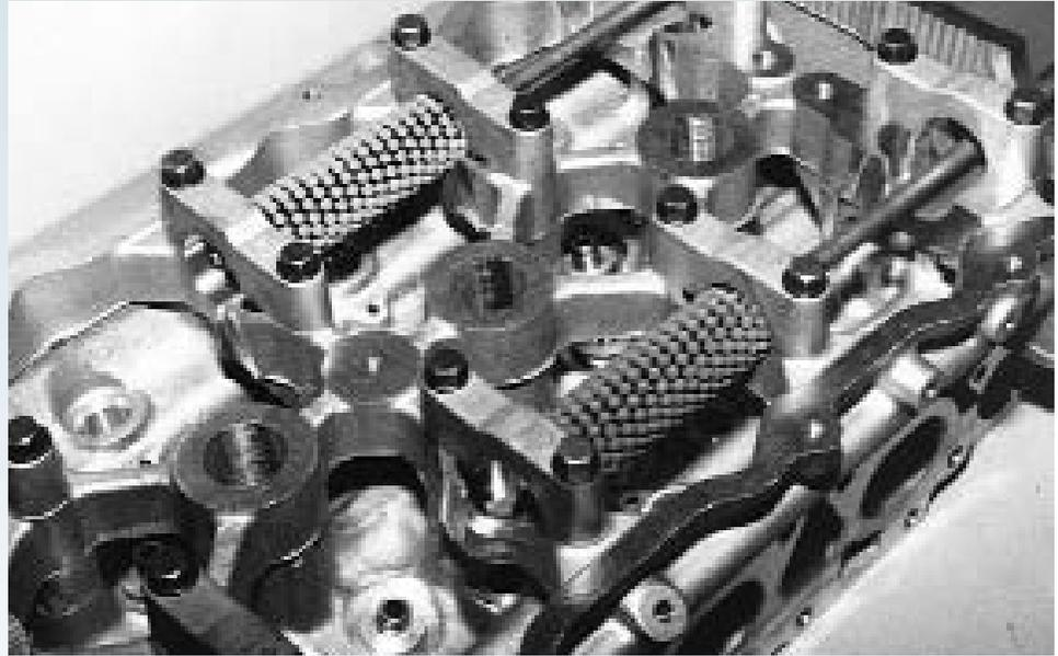
A resilient, flexible, honing tool with a soft cutting action. The abrasive (points) globules each have independent suspension that assures the Flex-Hone® to be self-centering, self-aligning to the bore, and self-compensating for wear.
